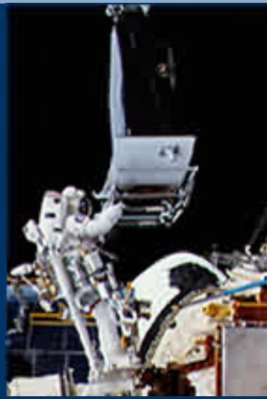
Astronaut Jeffrey Hoffman removing WFPC1 during changeout operations.
