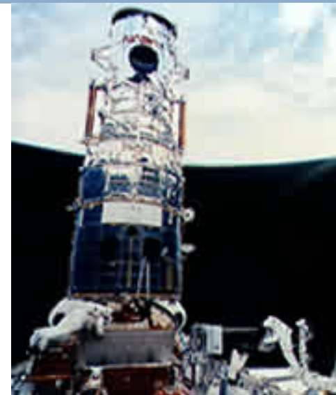
Astronaut Hoffman (right), anchored on the end of the RMS arm, holds onto WFPC1 during the third spacewalk.
