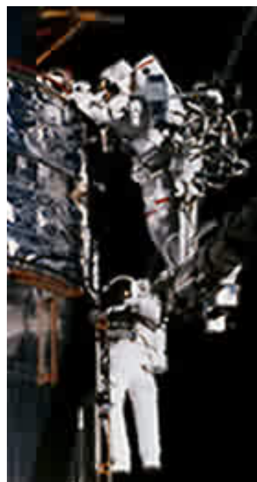
Astronaut Mark Lee (top) performs a patching task on Hubble's worn insulation material.
